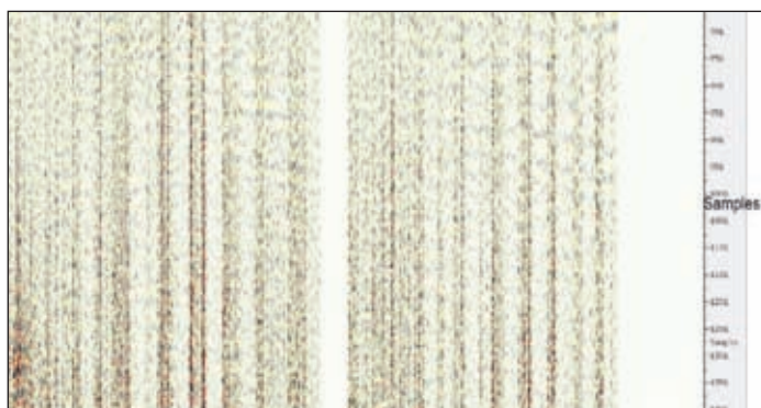
Fig. 9. Vibroseis to hydrophone, before noise removal.
